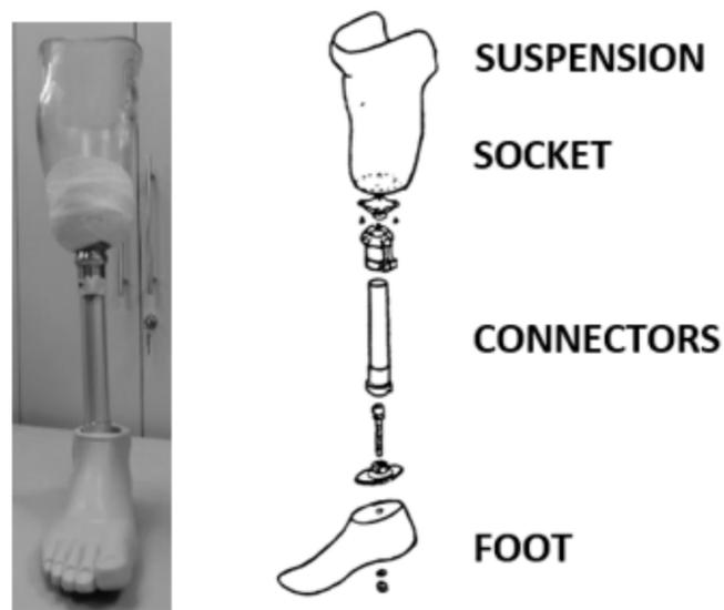
Fig. 1. Prosthesis used by amputees, suspension by liner and pin, and carbon foot of high activity.
