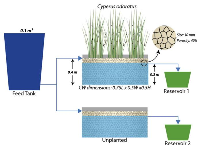
Fig. 1. Schematic representation of the pilot-scale industrial synthetic wastewater treatment plant using feed tank and SSF CWs (with *C. odoratus* and unplanted).
