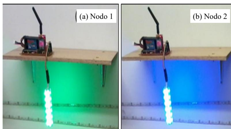
Fig. 5. ZigBee communication card with power module and RGB LED control.
