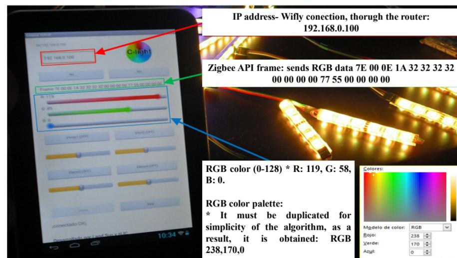
Fig. 9. APP Mobile cellular Control Wireless Network.
