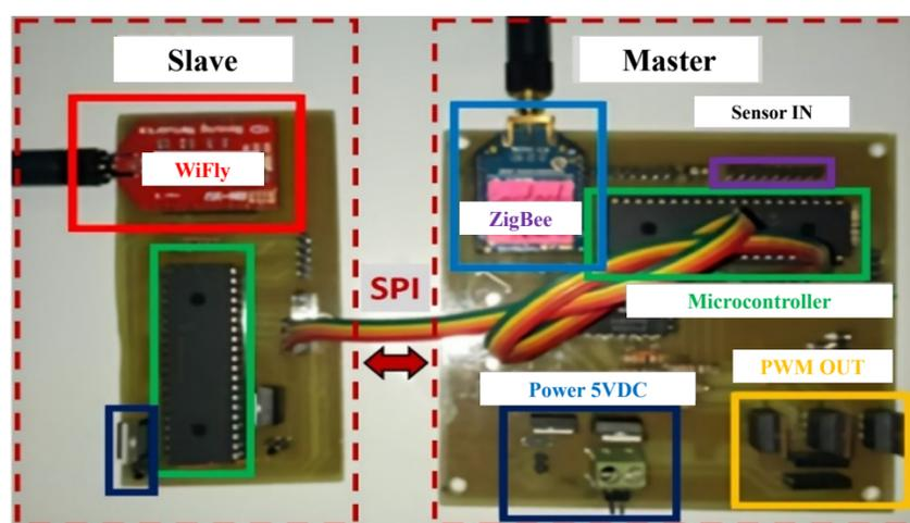
Fig. 1. ZigBee – Wifly Embedded System. Interconnectivity node.
