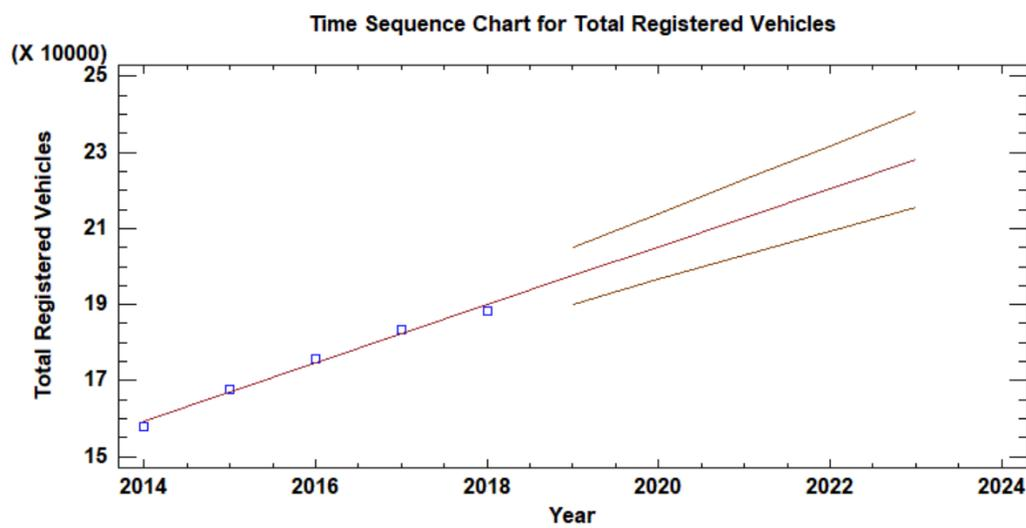
**Fig. 5.** Time Sequence Chart – Forecast for Total Registered Vehicles 2014-2023 in Barranquilla. Source: [6].
