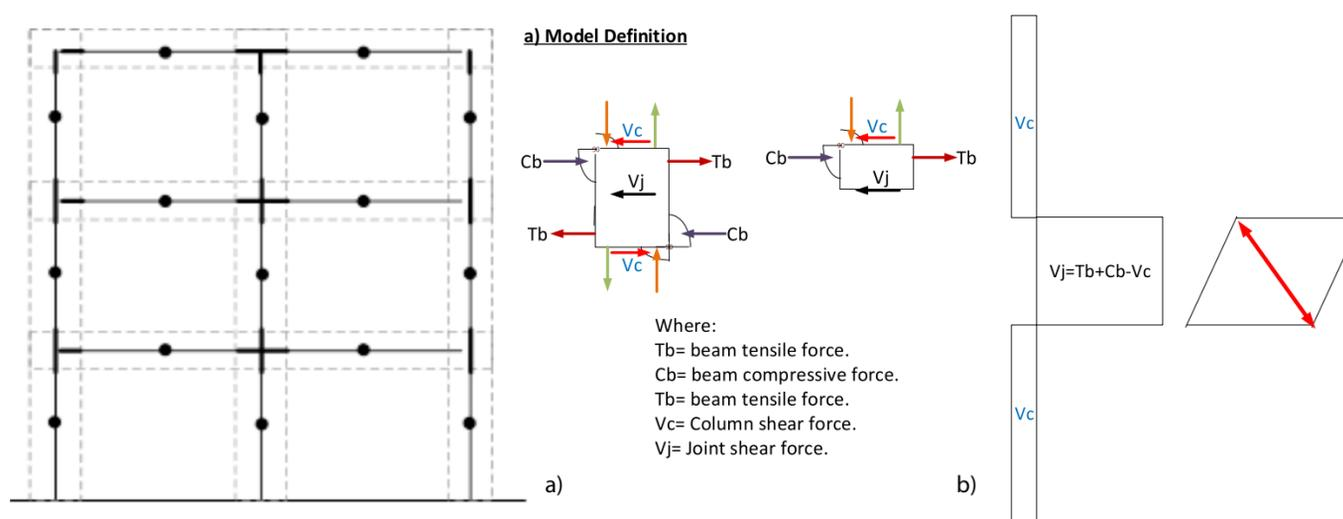
Fig. 1. BCJ idealization. a) Model idealization, b) Internal forces at BCJ, shear demand, and deformed shape.
