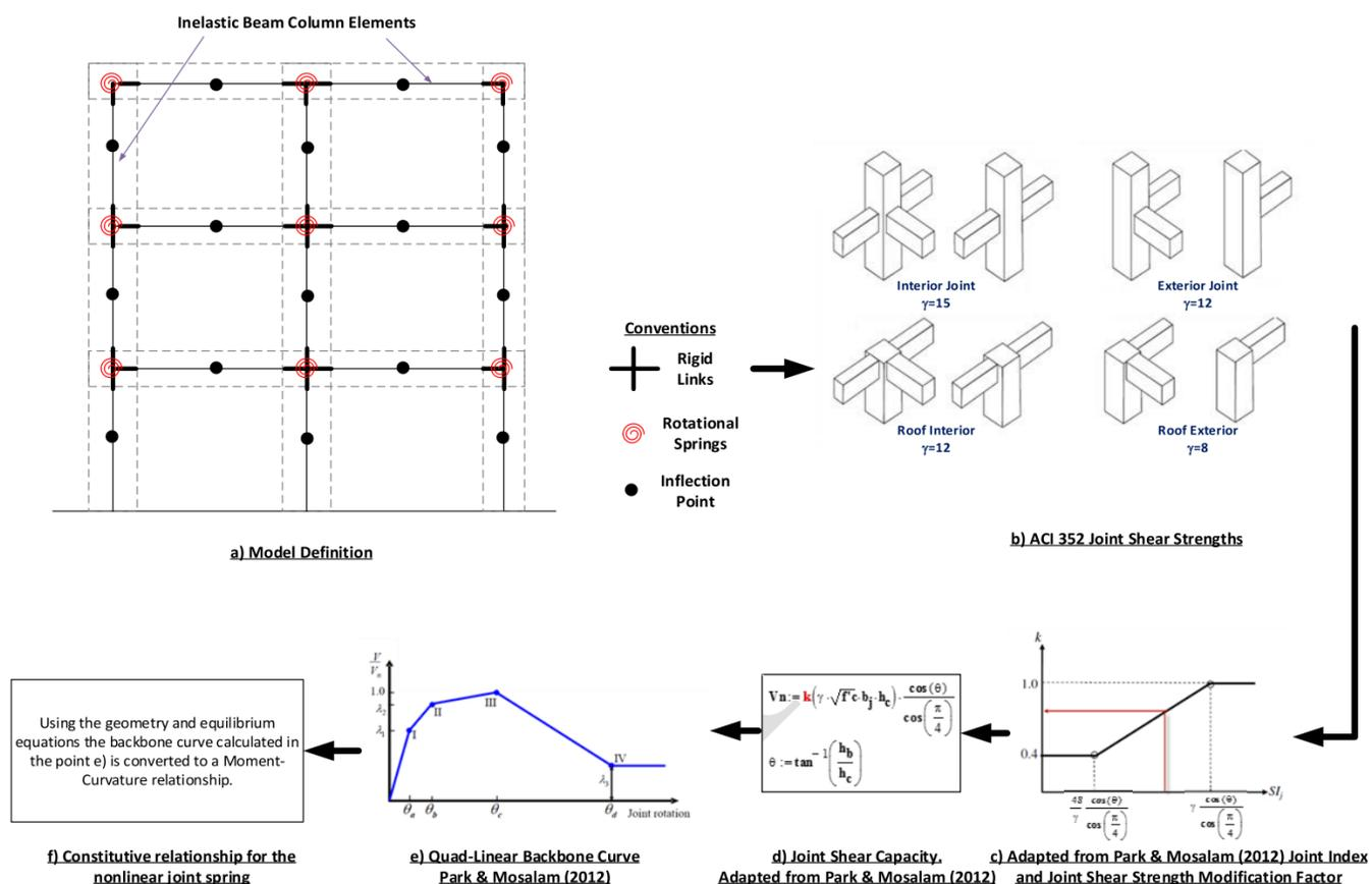
Fig. 5. Procedure outline proposed for modeling unreinforced BCJ. Source: Author adapted [50].
