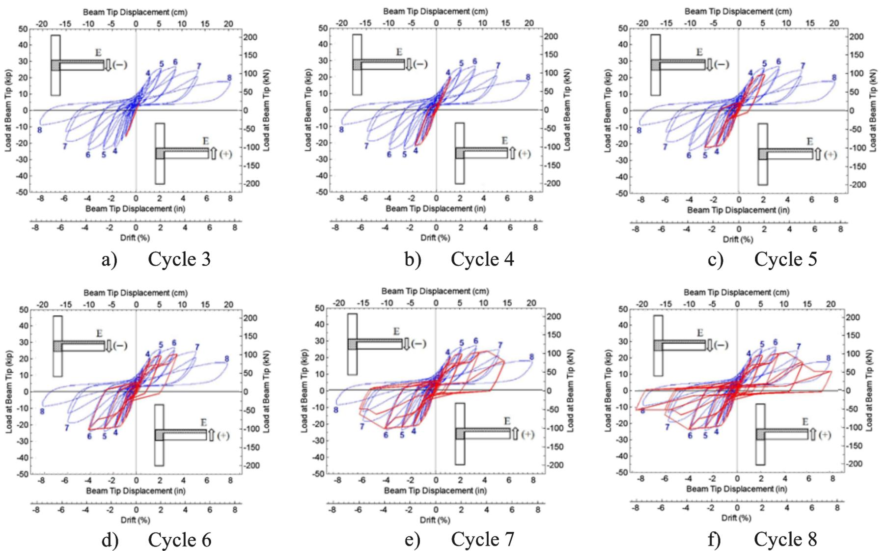
Fig. 6. Obtained load-displacement response SP1 EW.
