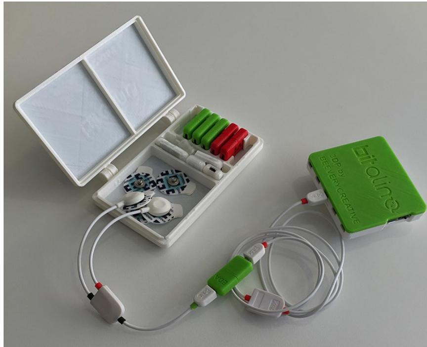
Figure 3. BITalino Acquisition Unit (plugged version).
