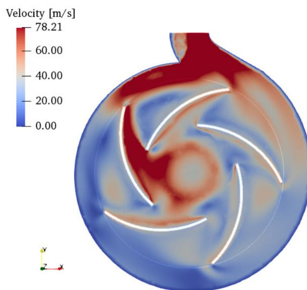
**Fig. 5.** Flow velocity simulated with RNGKEpsilon model.
