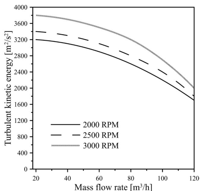
**Fig. 8.** Turbulent kinetic energy of centrifugal pump.
