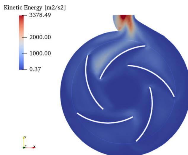
**Fig. 7.** Turbulent kinetic energy described with OpenFOAM.
