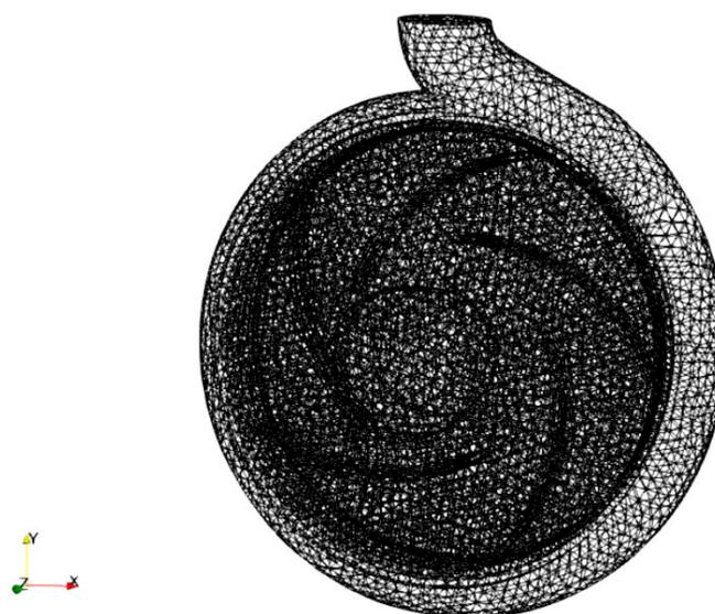
Fig. 2. Mesh density of computational domain.
