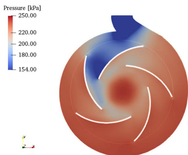
**Fig. 6.** Flow pressure simulated with RNGKEpsilon model.
