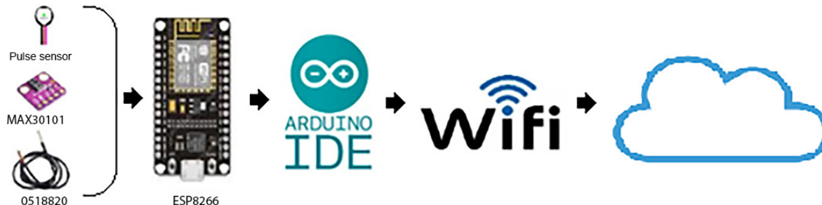
Fig. 1. Diagram of a prototype system for monitoring cardiovascular variables. Source: Authors.
